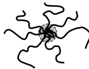
Figure 8. Star-branched microgel (shaded core) with semi-flexible rays. 39
